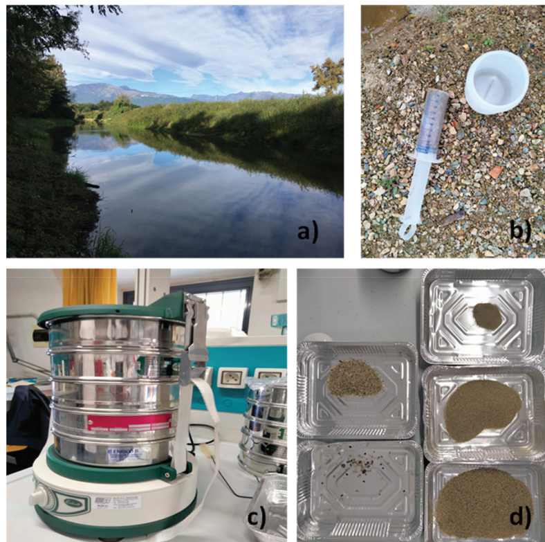
Figure 2. (a) Sampling station, Ghiandone River (NW Italy); (b) sediment cores; (c) Bertel mechanical sieve; (d) samples of the five granulometric classes considered.
